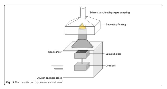
flaming occurred outside the test chamber, such that the amount of oxygen available to combustion exceeded the amount that was fed to the enclosed chamber.
