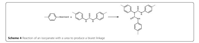
Short chains with high functionality results in highly cross-linked polyurethane polymers which is characteristic of rigid foams.
