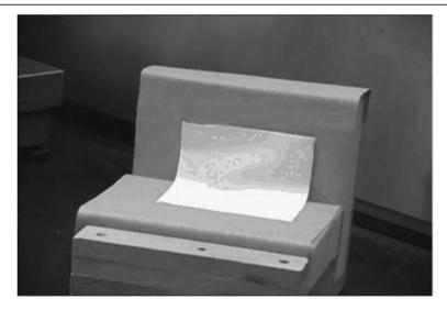
Figure 7 Mockup arrangement for UFAC smoldering ignition testing of barrier materials used in upholstered furniture.
