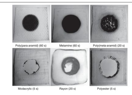
Figure 5 Char characteristics of nonwoven felts. Note: Values in parentheses show exposure time to open flame.
