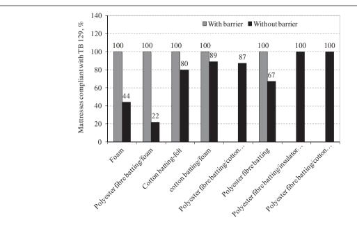
Figure 1 Comparison of full-scale flammability test results for innerspring mattresses with different types of filling materials in the presence or absence of fire barrier materials (Nurbakhsh & Mc Cormack 1998).
