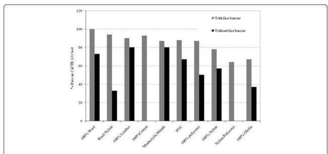
Figure 2 Impact of fire barrier fabrics on performance of upholstered chair (with different cover fabrics) in full-scale flammability testing (Damant & Nurbakhsh 1994).
