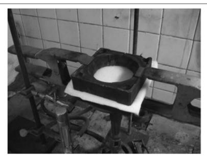
Figure 4 Meeker burner test set-up for studying char characteristics.
