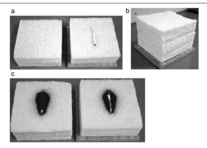
Figure 8 ASTM D 5238 test for smoldering ignition resistance of cotton batting: (a) start, (b) test in progress, and (c) end of the test. Cotton batting stack on left of (a) is placed on top of the cigarette/cotton batting stack on the right of (a) to form the testing setup in (b).
