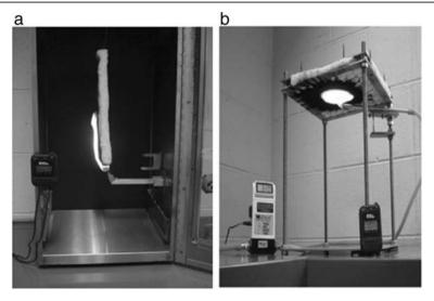
Figure 9 Modified Cal TB 117 for testing barrier flammability: (a) vertical and (b) horizontal configuration.
