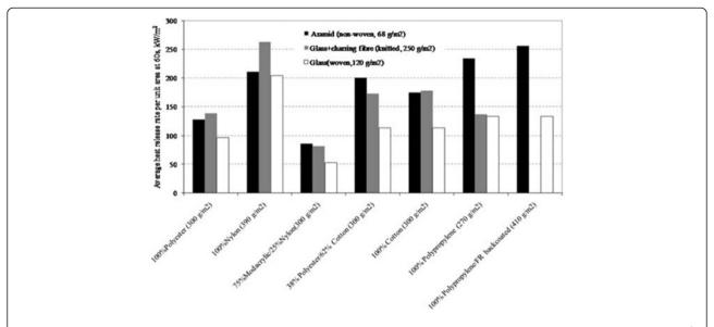
Figure 3 Impact of different cover fabrics and fire barriers on PHRR of composite specimens tested under cone calorimeter (35 kW/m<sup>2</sup>) (Ohlemiller & Shields 1995).
